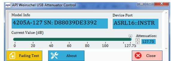
Spectrum Control's Weinschel LabView based USB Control Center Software (AUCS) can also be used in the operation of this series of digital attenuators. The AUCS will allow the user to setup, control, and perform test and measurements over a standard USB 2.0 communication interface. Additional information is available in the Operating & Installation Manual, IM-611.
