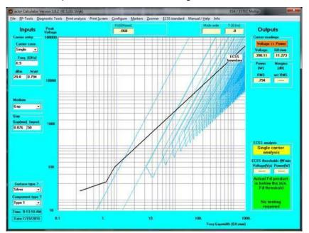
Highly specialized multipactor predictive tools enable filter and other RF passive component designs that ensure a long life of operation without concern of this breakdown threat.
