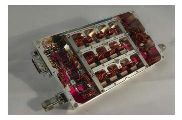
Assembly chassis for high power SFBs must be designed to incorporate design elements to optimize electrical, RF, and thermal performance.
