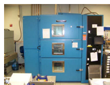
Extensive Burn-in and Thermal Cycling Capabilities
