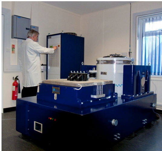
Figure 3 Vibration Test Equipment
